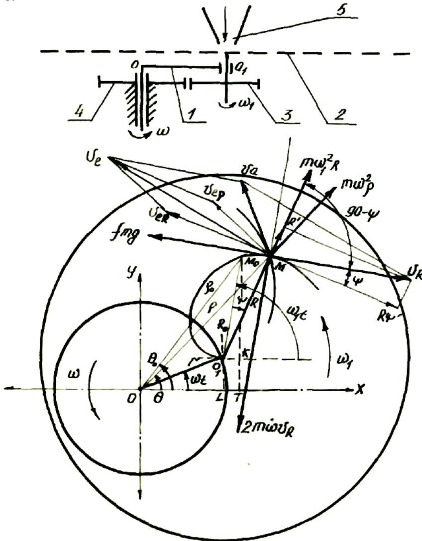
Figure 2. Sieves with a sun and planet motion.
