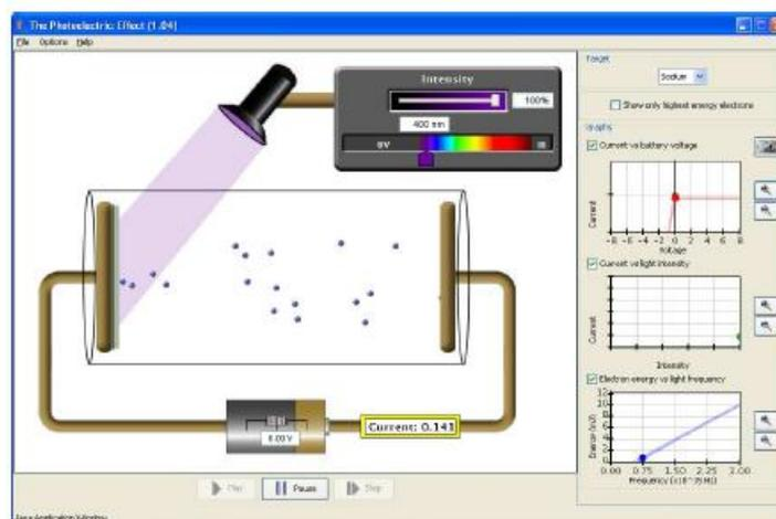
**Figure 2.** The Photoelectric Effect simulation (Color online)
