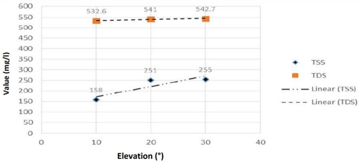
**Figure 7.** Relationship of TDS & TSS values with Filter Position Slope
