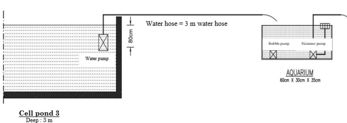
Figure 5. Laboratory Scale Flocculation Method
