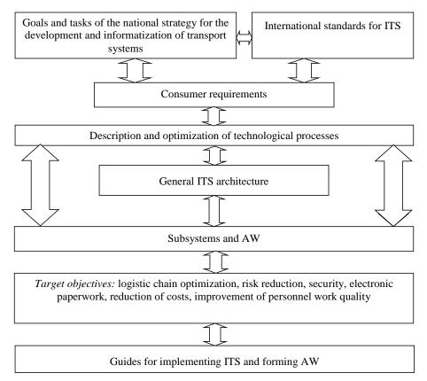
Figure 2. Intelligent transport system model
