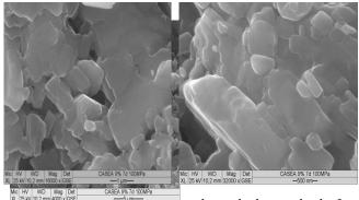
Figure 5. Merging of gypsum particles of the pressed samples (conditions: ground natural gypsum, pressure of compaction 100 MPa, water-gypsum ratio -0,09, storage in closed containers - 7 days)
