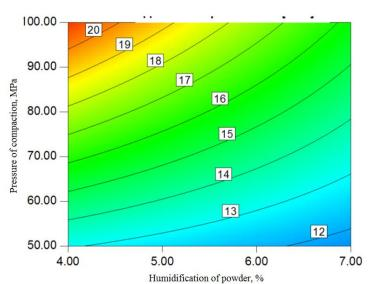
**Figure 4.** The strength at compaction of the samples from the pressed gypsum particles depending on the moisture content of the material and pressure of compaction (test conditions: storage temperature of samples: 20 °C, storage time: 7 days, without the use of a plasticizer)
