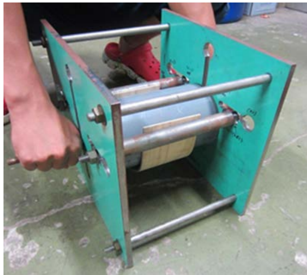
Figure 17. Apparatus of bending processing test
