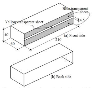
Figure 2. Dimensions (in millimeters) of the device used to furnish a guide line for the reading from the chalkboard
