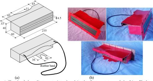
Figure 4. a) Sketch of the adjustments introduced in the first prototype of the Line Finder. Presented dimensions in millimeters; b) The second prototype, with improvements to hold the transparent foils and reinforcements of the supports. The main dimensions are the same of Figures 2 and 4a
