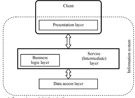
Figure 1. Program layers of distributed software
